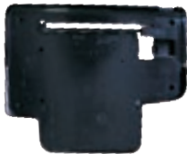
Small Top Cover Material:PC+ABS+FR40 Weight:350G Thickness:2.0mm Nozzle type:SSV 25 VV
