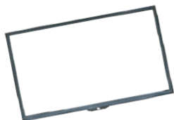
TV Front cover(32") Material:PC+ABS+15%GF Weight:158G Thickness:2.5mm Nozzle type:12-PSM 18 VV
